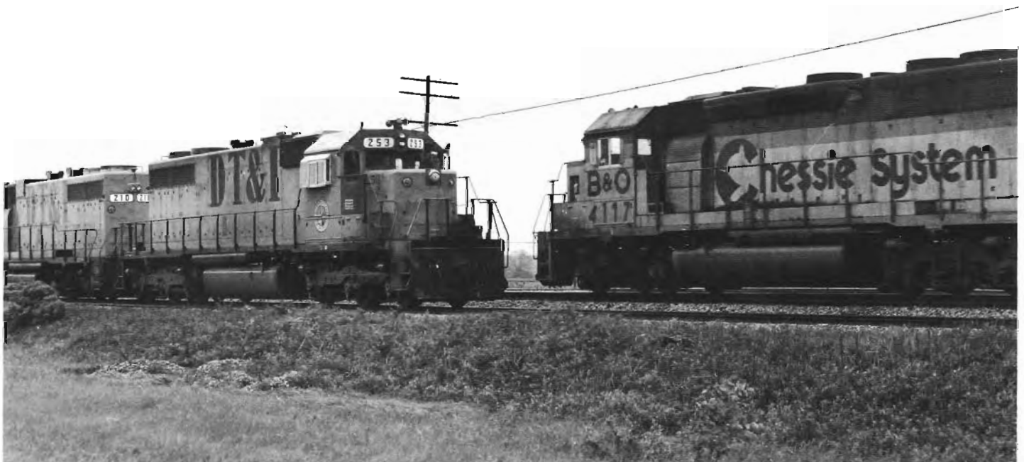
Above - An SD-38 and GP-38 are stopped on the passing siding at Ottawa, Ohio as a northbound B&O grain train with an original Chessie unit (extra large cab initials and silver trucks) blows by at 50-mph.
