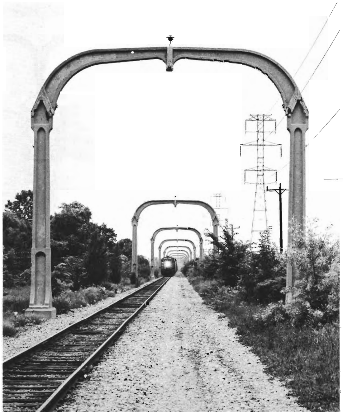
A northbound puller, powered by GP-38 #203, travels under Henry Ford's catenary arches at Taylor, MI in June, 1979.
