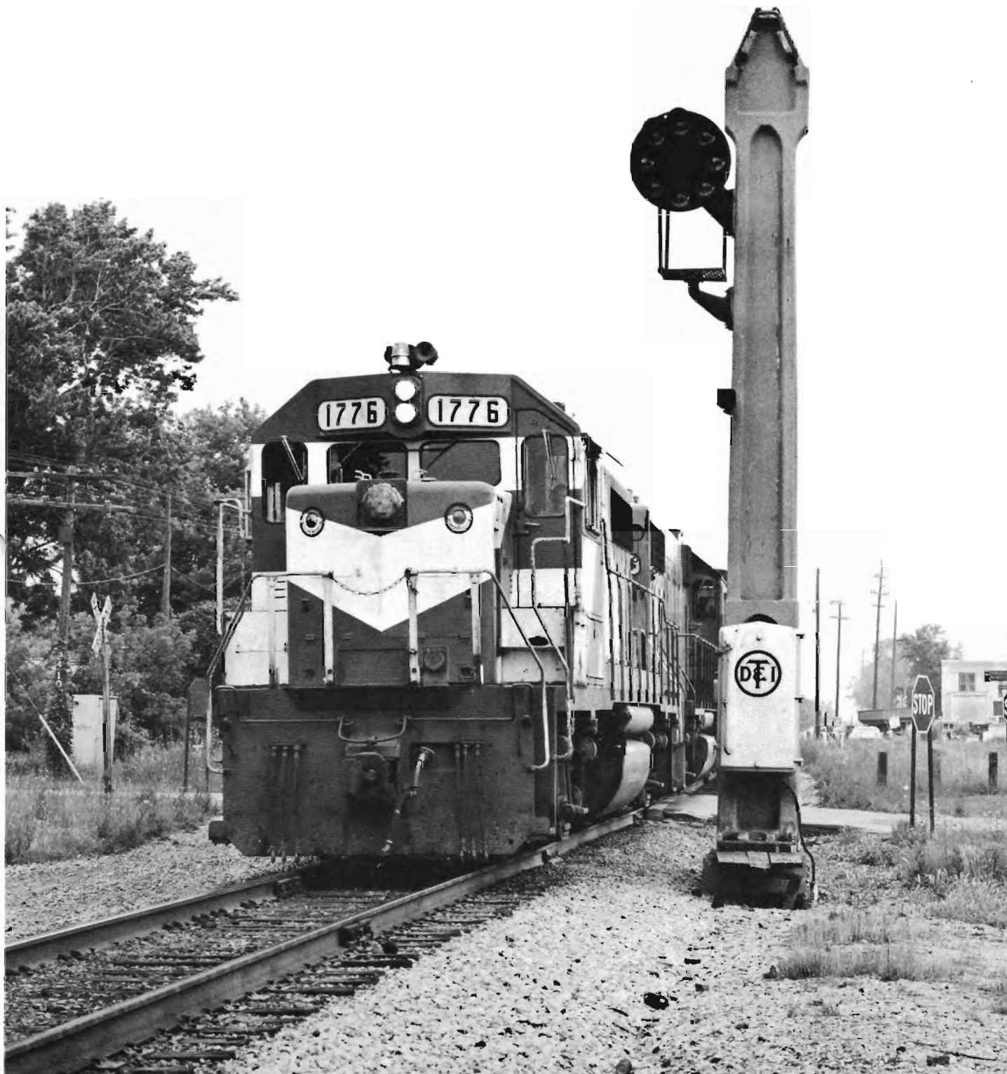
Symbol freight DS-3 with lead unit 1776 still in its Bicentennial livery (it has since been repainted and renumbered to 228) rolls past one of the few remaining remnants of the great electrification project still evident south of Flat Rock. The location is Carleton, MI, and the old pole survived to serve double duty as a signal post. Note the old DT&I herald on the phone box. That emblem was superseded by the DT&I's compass emblem about 1954.
