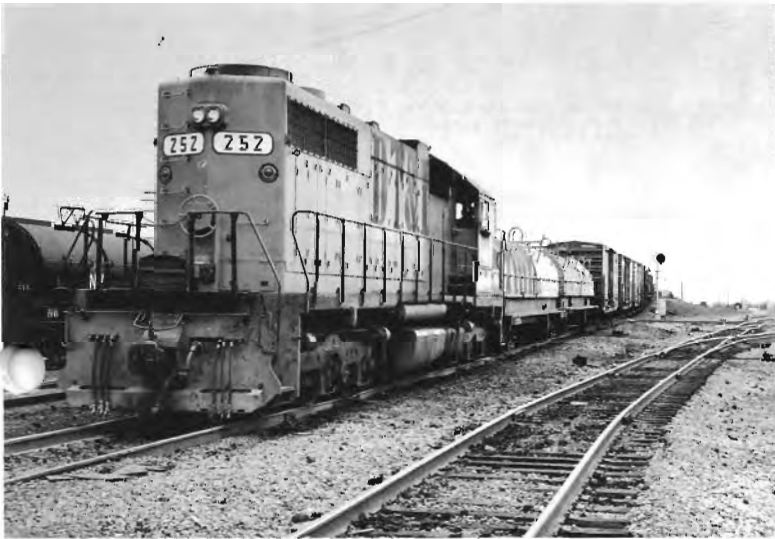
The 2,000 horses inside #252's body are harnessed to work the Flat rock hump in 1979.
